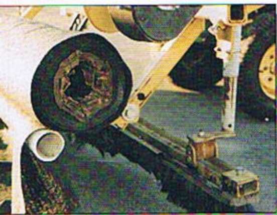
Poor storage results in wet cores, which creates installation problems.
