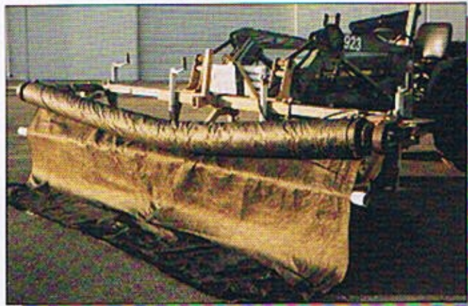
Fabric on cores that are too light cause rolls to sag in the middle, creating installation problems.
