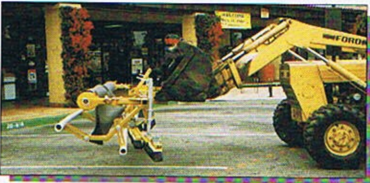
Proper placement of fabric roll on placement machine on a front-end loader.
