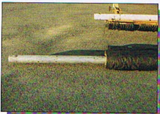
Reinforcing cores using aluminum or steel pipe can make damaged cores easier to use.
